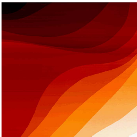
FIG. 2. (Color online) STM topography image of an 800 \times 800 \text{ nm}^2 Ag(111) surface. Tunneling conditions are U_{\text{sample}} = -1.70 V and I_t = 95 pA.
